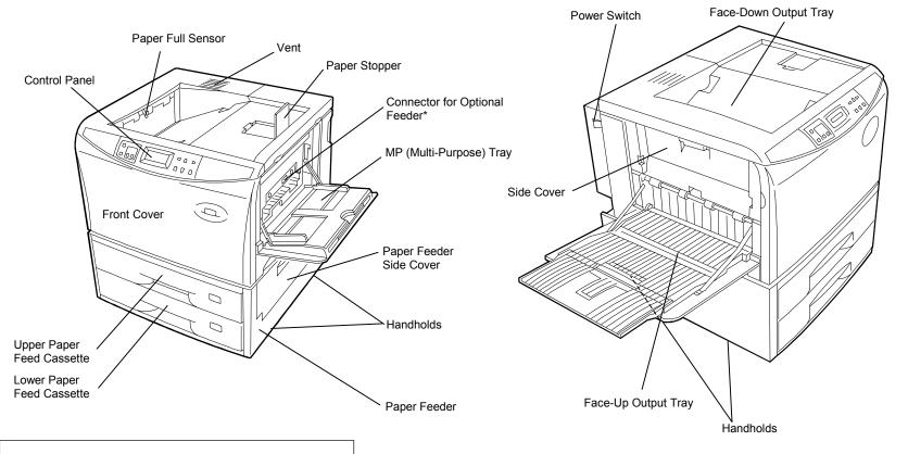
\* To prevent static electricity, be sure to cover the optional feeder connector not being used with the protective caps supplied with the printer.
